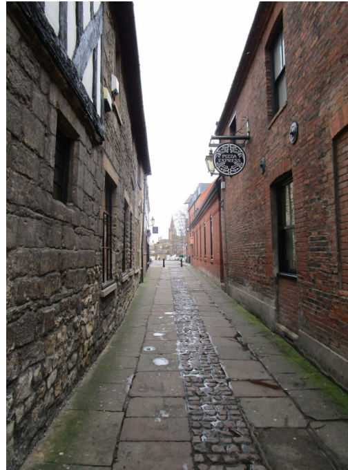
Plate 44 Ginnel from High St to Grantham St showing stone flag and sett surfacing.
